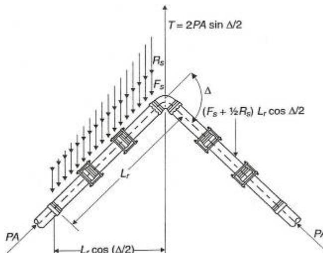
**Figure 5: Resultant Frictional and Passive Pressure Forces on a Pipe Bend**
