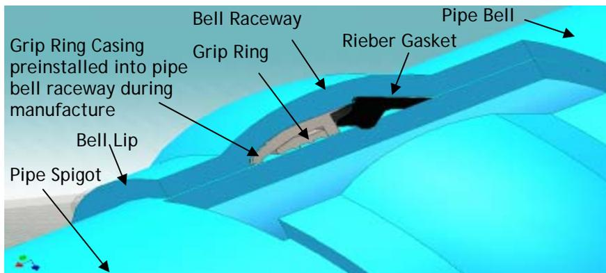
**Figure 7: Cross Section of Installed BullDog™ Joint**
