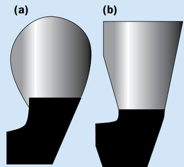
ter elastomeric gasket functions is shown in Figure 5. In the absence of internal pressure, a compression seal is formed as the elastomer is squeezed between the bell and spigot. Under internal pressure, the elastomeric material is redistributed and pushed forward within the pipe-bell recess. The higher durometer elastomer ensures the seal is firmly seated within the bell recess and that blowouts don't occur; leakage is prevented by compression sealing of the lower durometer elastomer.
