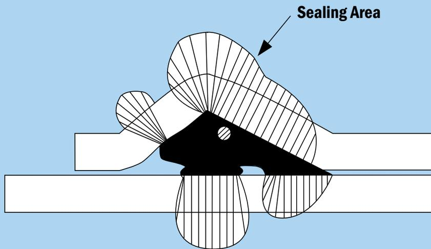
were finally resolved with the introduction of the Rieber-type gasket in the late 1970s. Today, more than 90 percent of PVC pipes in North America use the Rieber joint while less than 10 percent use the dual-durometer type. Rieber is a generic name used to describe a steel-reinforced elastomeric seal that is incorporated in the pipe bell during manufacture, making the gasket an integral part of the pipe.
